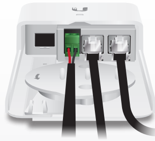
24/50V DC Output 24/50V DC Input 24/50V Power and Data to PoE Device
